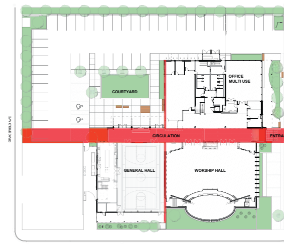
Site and ground floor plan illustrating the design concept of a cross laid down on the site
