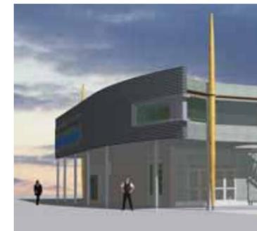
The choice of corrugated steel material and dark colour, is a metaphor for the Trusts flagship, a barquentine, the "Spirit of New Zealand," which moors on Princes Wharf, immediately in front of the new building. The texture of corrugate is suggestive of the original clinker hull construction of old sailing vessels, and the ship is black.
