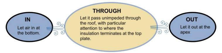
That is the normal passage of water vapour on a still night. It may be reversed due to wind conditions, but the principle remains the same.
