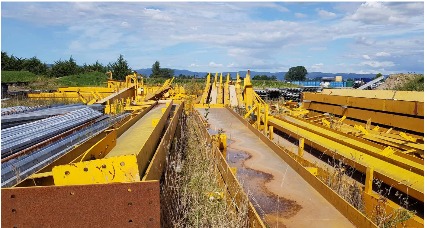
Stored, recycled steel awaiting re-use.
