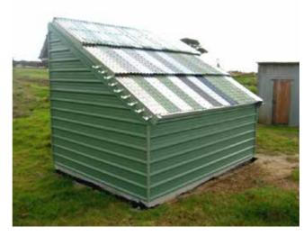
This was done by building special sheds with 45 degree roofs with three rows of panels, eight different substrates and 8 different screws.
