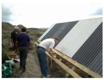
Roofs for tiles. Into this roof screw suppliers installed a range of their screws as they would normally have supplied.
