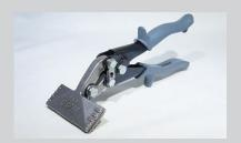
Hand Seamers are used to hand fold small flashings, by progressively working along the edge of a sheet.
