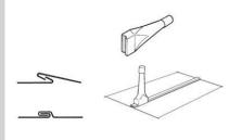
All metal joints that are to be sealed should be mechanically joined. Seaming is one acceptable method of joining two pieces of metal.
